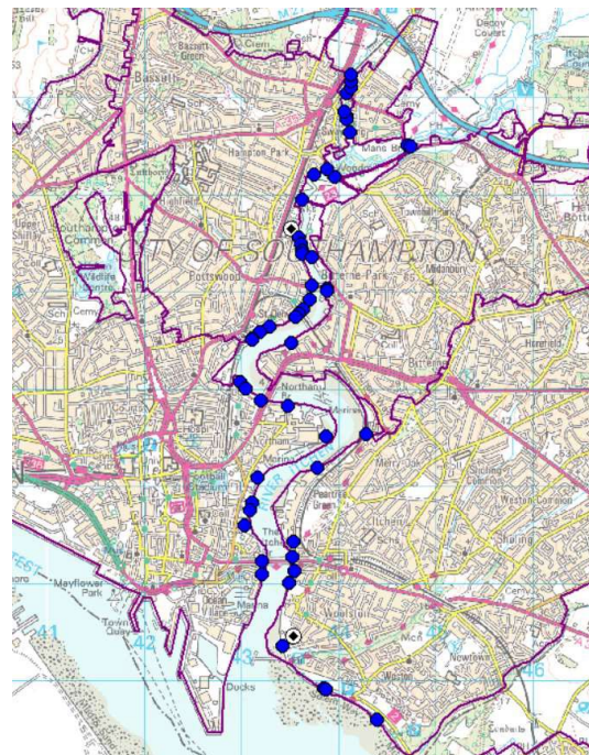
Figure 8 - The location of surface water outfalls into, and near to, the River Itchen in Southampton
